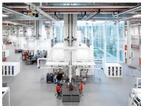
04 In the hall, the type chosen features four LED arrays, neutral white colour temperature and wide beam light distribution. In this version, the floodlight generates a gross luminous flux of 27,760 lumen at 212 watts of system power.
